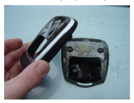
Getting the inside of the lock out of the space is a bit tricky as the linkage gets in the way but a minute of fiddling and out it comes.
