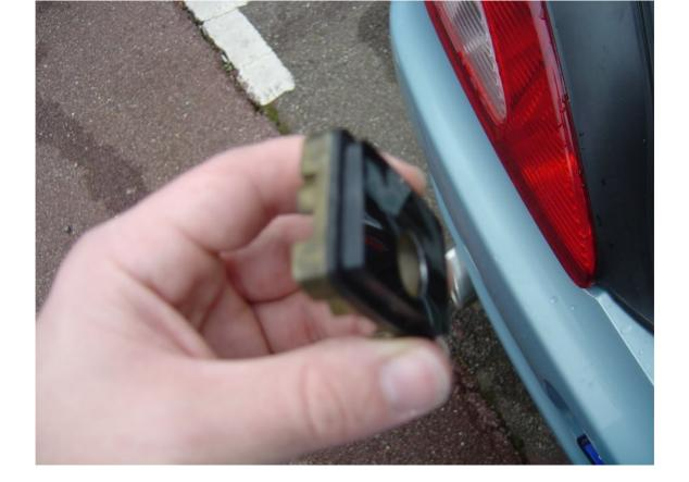
But if you're careful you can prise off the fascia and replace it on your old lock therefore removing the need to dismantle the lock.
