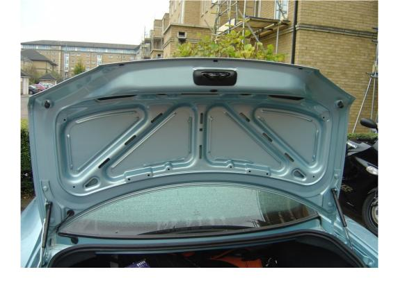
Next I removed the catch (two T30 torx screws) and you'll need to take out the rubber grommet circled in red.
